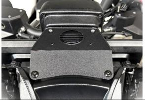
Install the radar display to the dashboard using the screws provided by the radar company for the installation.
